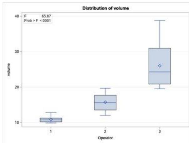
**FIGURE 4.** Volume (mm<sup>3</sup>) of tooth structure removed during post removal. Group 1: resident robot guided, Group 2: experienced FH, Group 3: resident FH
