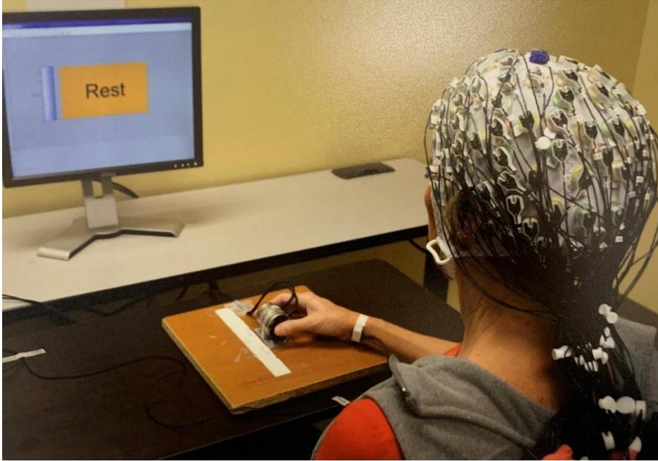
**Figure 1.** Experimental setup for the EEG grip task.
