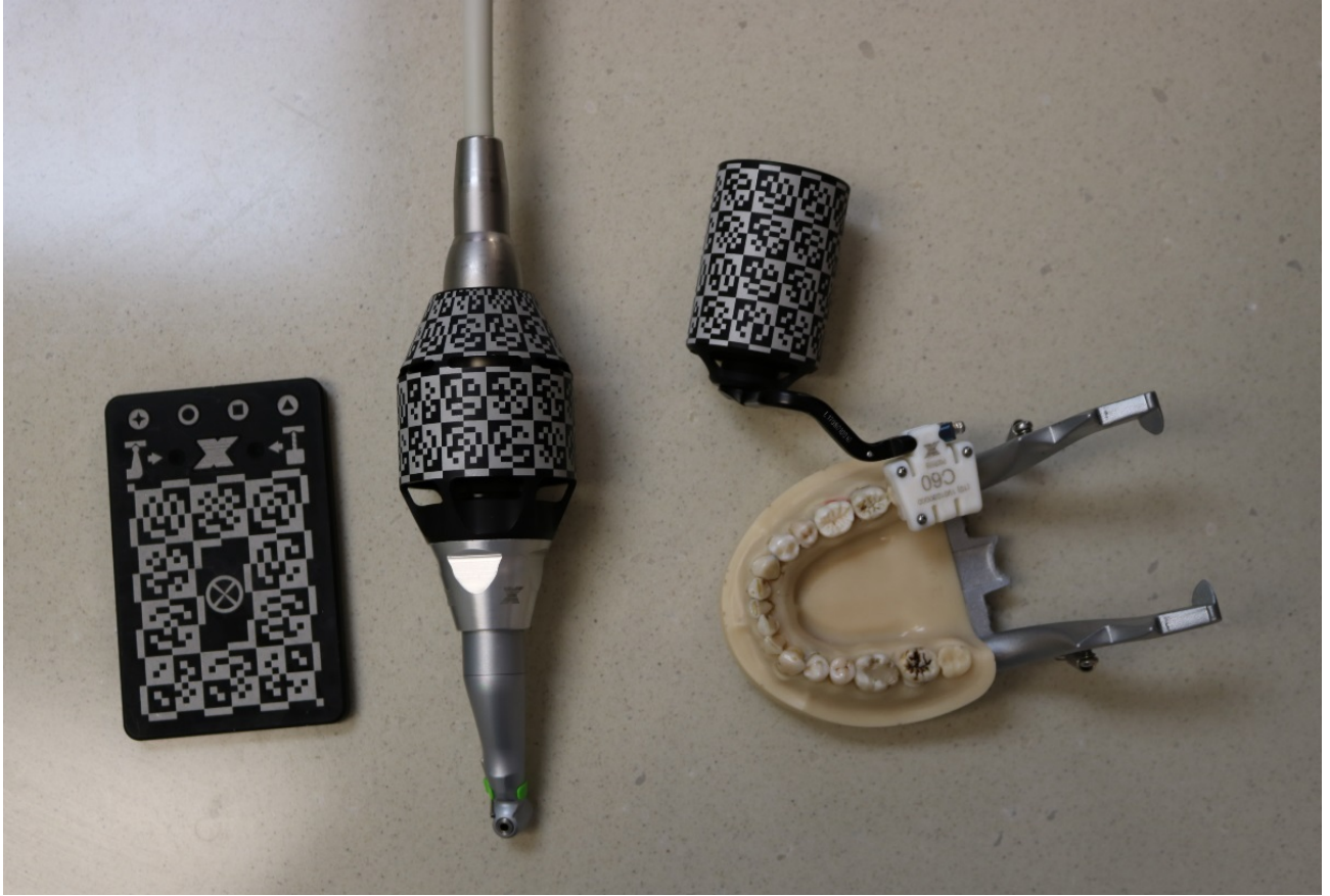
Figure 5. X-Guide sensor plate and dynamic reference frames used for system calibration and tracking. From left to right: bur sensor plate, hand-piece DRF, and patient DRF.
